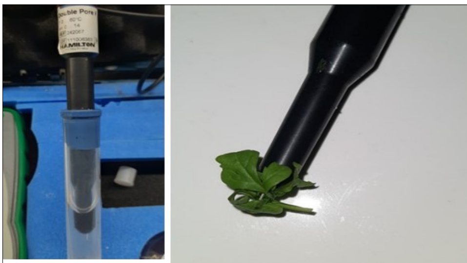
Figure 2. Measuring the foliar pH
